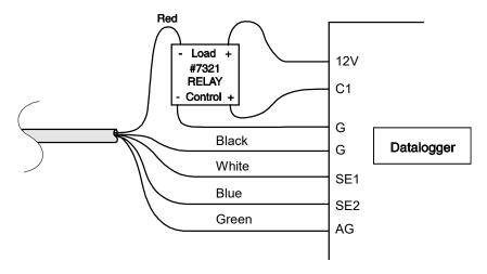
FIGURE D-1. Wiring diagram for connecting an OBS sensor to an external relay and a data logger
