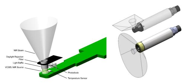
FIGURE 5-1. Components of the OBS-3+ (left) and orientation source beam and detector acceptance cone of the OBS-3+ (top right) and OBS300 (bottom right)
