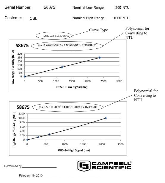
FIGURE 7-2. Calibration certificate showing millivolt coefficients
