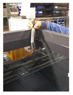
FIGURE 8-2. Position of OBS-3+ (left) and OBS300 (right) in clean tap water in big black tub
