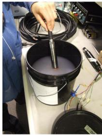
FIGURE 8-3. OBS-3+ (left) and OBS300 (right) in 500-NTU AMCO Clear® turbidity standard in 100-mm black polyethylene calibration cup
